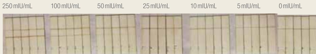
**Figure 7:** Anteo magnetic particle test strips run with hCG diluted with urine.
