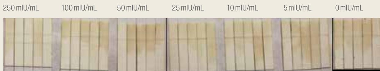
**Figure 8:** Covalently conjugated magnetic particle test strips run with hCG diluted with urine.
