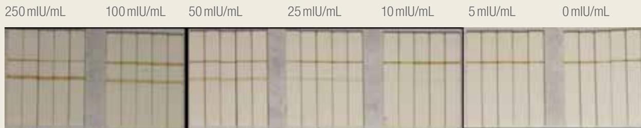
**Figure 3:** Anteo magnetic particle test strips run with hCG diluted in buffer
