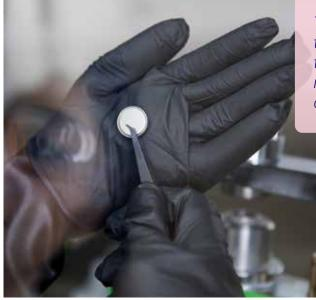
$\label{thm:condition} \mbox{AnteoTech's coin cell battery, incorporating the High Silicon Anode ready for } \mbox{\cite{thm:conditions}} \mbox{\cite{thm:condit$
